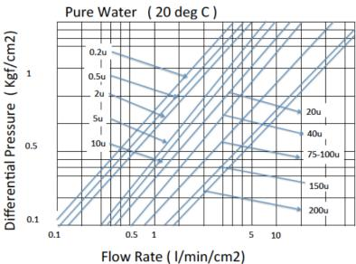
Pressure Drop with water / 10" length cartridge
