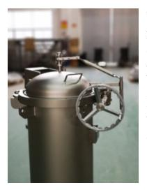
There is a handle that linked to the pressure relief valve need to be in lock position for complete close operation during filtration process.
