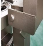
With the help of spring balancer incorporated in our filter vessel design, operator can easier lift up the cover and rest on at 110 deg position, there is a safety pin to lock the cover arm for safety precaution consideration to prevent the cover from dropping down
