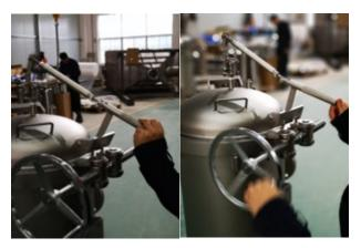
After filtration for changing of filter bag, the operator first needs to open the pressure relief valve by lifting up the handle in order to operate the spindle to release the cover.
