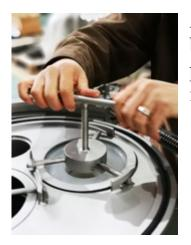
After changing the filter bag, each bag need to b securely lock with cover ring by using a tool provided to ensure each bag are properly installed, no by pass allowed.
