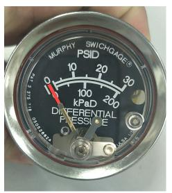
Differential Pressure gauge for you to set the differential pressure to perform cleaning operation, recommend to set at 10 psid.
